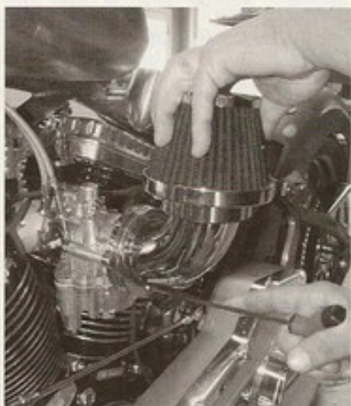
25 Air supply duties will be handled by this chrome Wimmer updraft air cleaner assembly.
