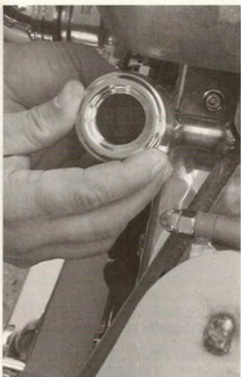
27 After welding a Dakota Digital gauge nacelle to the left side of the frame, Scott pops in a chrome Dakota Digital LED speedo. The gauge will get its signals from a Biker's Choice speedo pickup in the Rivera six-speed transmission.
