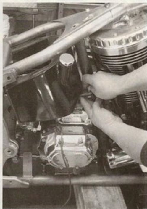
2 The first parts on this month are a Paughco wraparound oil tank, which is supported by a Biker's Choice oil tank mount.
