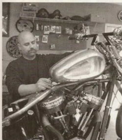
22 This dished Paughco gas tank will do a great job of keeping the V-Plus engine's fuel supply safe while looking cool.
