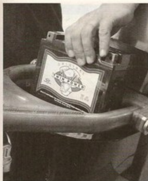
21 A Biker's Choice battery, battery strap, and battery cables will supply our bobber with the electrons it needs to run.
