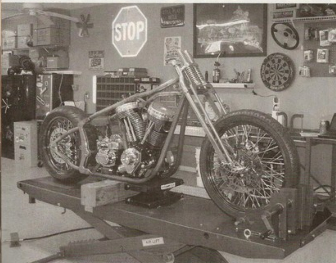
2 The first parts on this month are a Paughco wraparound oil tank, which is supported by a Biker's Choice oil tank mount.
