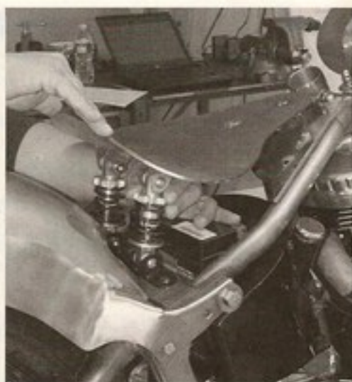
24 A Chopper Shox seat pan and seat shocks builder's kit will see to it that the rider's butt is happy whenever it's in this saddle! This pan will be covered by Alligator Bob at Advanced Custom Design.
